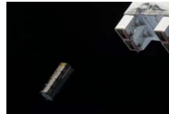
"TuPOD" deployed from the JEM Small Satellite Orbital Deployer (J-SSOD) Credit: JAXA/NASA®
