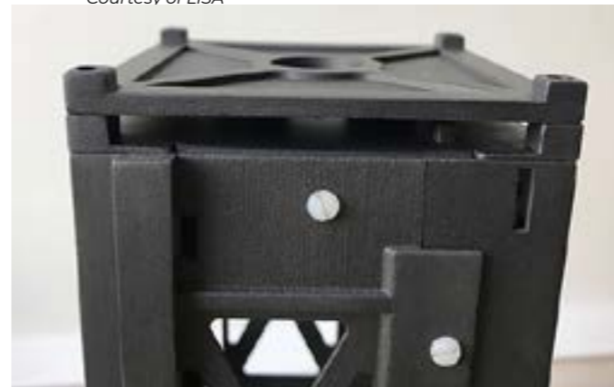
Antenna frame integrated in the 3D printed structure. Courtesy of LISA
