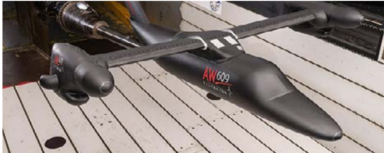
Model installed in the 11' x 11' test section at NASA Ames. Courtesy of LEONARDO HD
